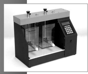
The PB-980™-Series Two-Paddle JarTester's small size makes it an ideal tool for Chemical Sales Reps to demonstrate the effectiveness of their coagulants. The programmable version, outfitted with B-Ker²® Lab Jars, is pictured at left.
